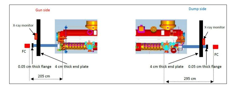
CMTB and AMTF have only two X-Ray detectors located at both ends of cryomodule: 'GUN side' and 'DUMP side'.
