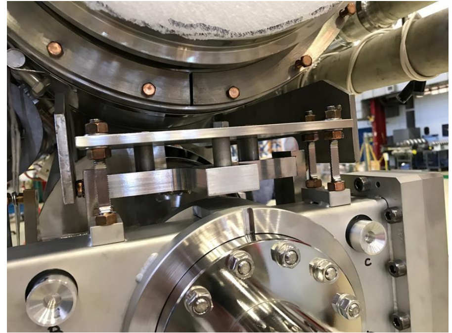
Flex configuration (spool between Cav#1 and valve) gate valve support frame installed on F1.3-4 and F1.3-5 (installed to a completed CM)
