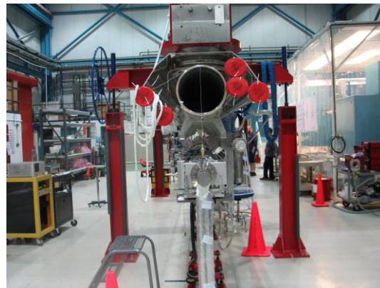
Upper Cold Mass to string alignment
