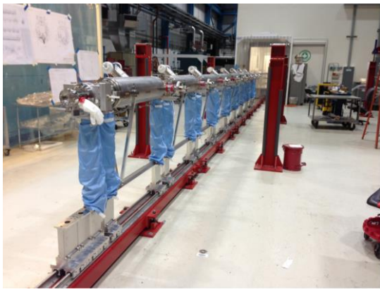
Cavity String on cleanroom assembly tooling rolled to WS2
