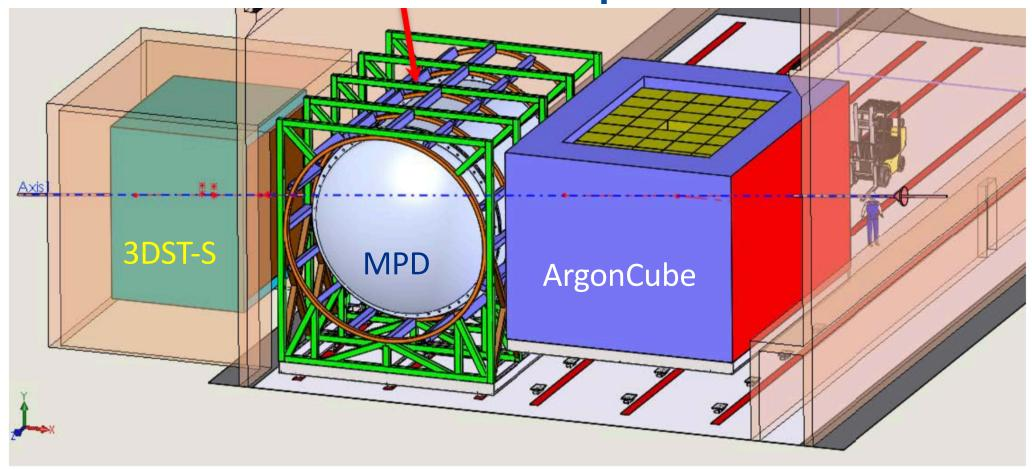
ArgonCube: Pixel-based LArTPC, unmagnetized (150 Tons)
