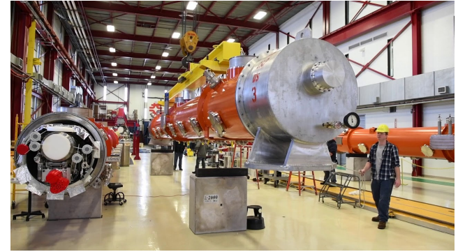
Cryomodule built at Fermilab for the new LCLS-II free electron laser light source at SLAC
