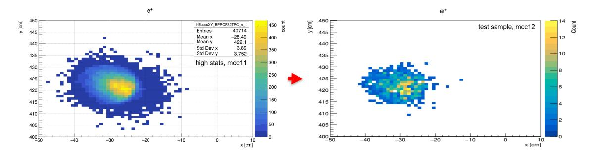
Beam spot still appears to be asymmetric around beamplug
