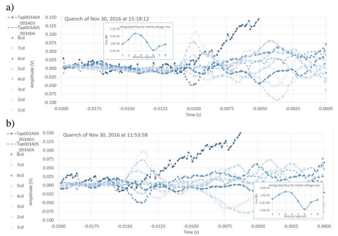
Fig. 8 Example quenches with voltage tap and quench antenna signal, both with a similar quench pattern. Quenches occur in the same coil 03. The insert shows the integrated flux during the initial antenna voltage signal rise, used to localize the quench, as explained in the Introduction and Fig 1b).
