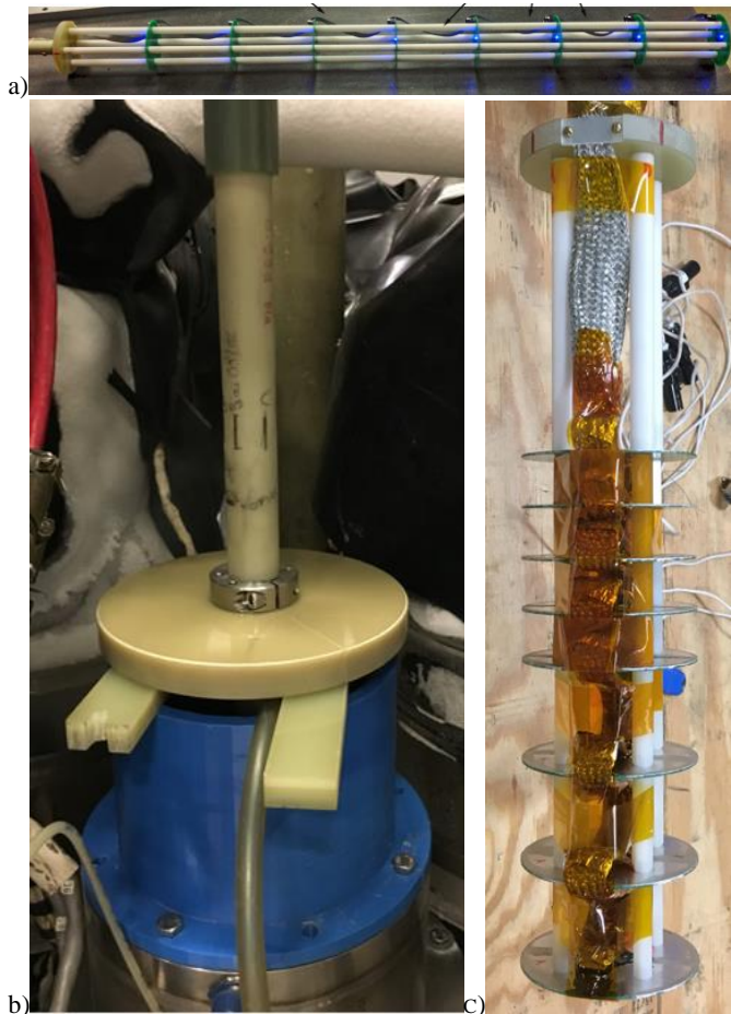
Fig. 3. a) A photograph of the quench antenna at 107.1 cm length, b) A photograph of the warm top with the clamped quench antenna rod. c) A picture of the shortened quench antenna with 5 segments at 2.54 cm spacing, and three segments with 5.08 cm spacing.
