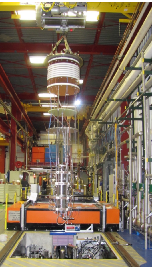
Fermilab Vertical Test Stand used for cryogenic tests of accelerator SRF cavities
