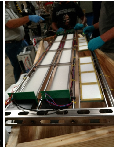
CERN test of dipped acrylic bars and dichroic filters (all made at FNAL)
