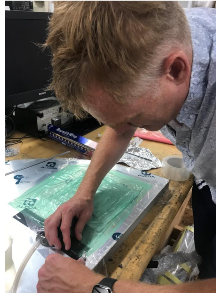
Removing bagging materials
