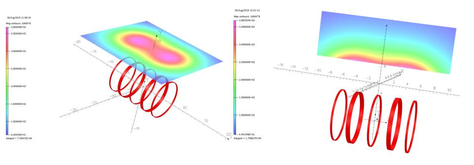
Fringe fields less than 370 Gauss shown as zone maps at the distance 8.4 m from the magnet center where the cryogenic equipment might be placed.
