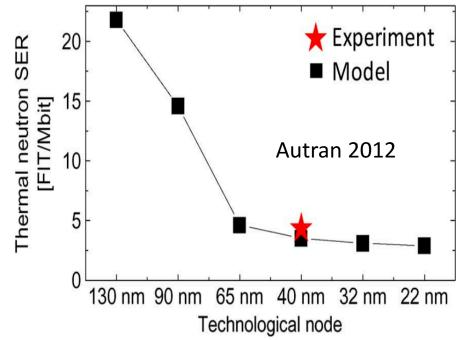
Autran (2012) used atmospheric neutron spectrum of NYC (US DHS) < 1eV and PROMO40v5 test chip by STMicroelectronics
