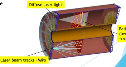
Pattern of Al dots (low work function →release of e-'s)
