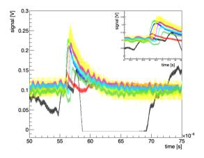
$\Rightarrow$  The relative difference of the onset of each shortening-cards signal allows to establish the track inclination angle
