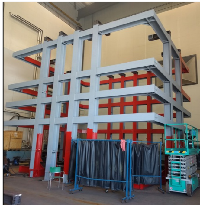
Warm cryostat structure construction at Cern
