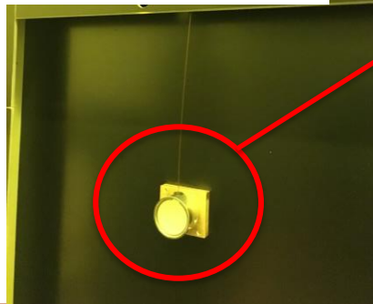
Pictures of light diffusers and fibers integrated with one CPAs at CERN.
