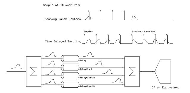
• 1200 MHzSampler bandwidth resolves high frequency structure on beam (pickups?)
