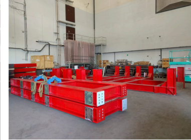
July 15 th Painting and trial assembly completed. Getting ready for shipping
