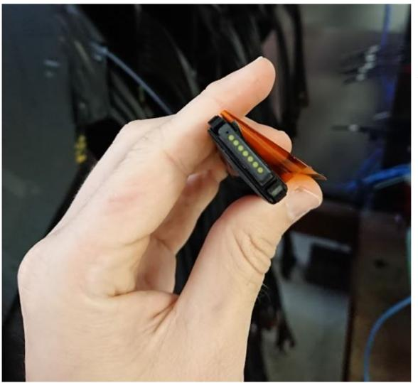
In assembly cleaning was done with ethanol and q-tip
