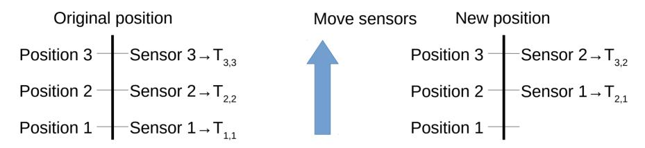
Assuming constant temperature during process, calibration constants can be computed as  $T_{2,2}$ - $T_{2,1}$  or  $T_{3,3}$ - $T_{3,2}$ .
