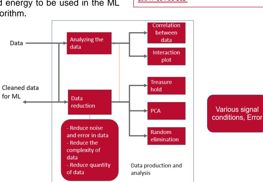
The data are produced by simulation or gathered from test facilities. It is the analyzed by plotting features vs other features to see how data are distributed in the parametric space. Different metrics can be implemented to test the data. The data size is also filtered to reduce noise and error, complexity, and the large quantity of data. After each elimination of data, the data are analyzed again to evaluate quality.
