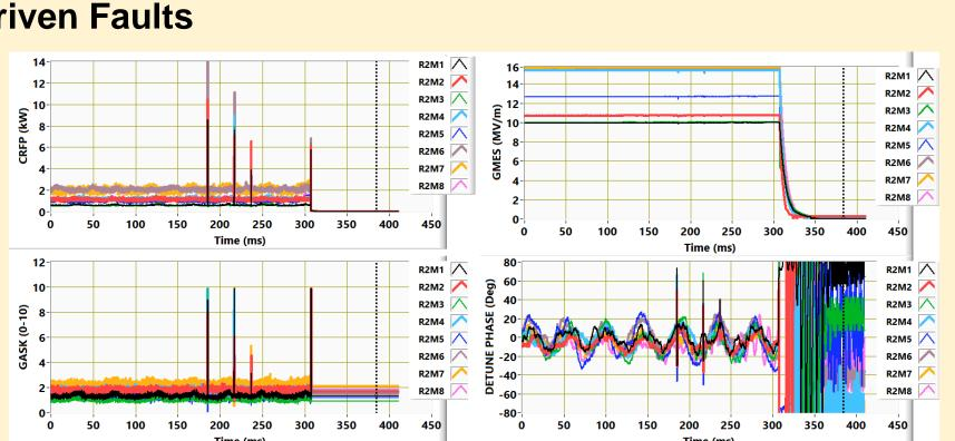
Single event (50 us sample rate) errors which occur in the south linac during thunderstorms. It is suspected that it is a grounding problem associated with either the MO or LO distribution system.
