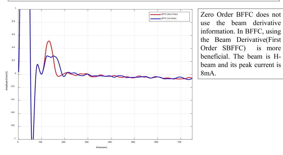
In order to test the performance of the ILC in case of multi-beams, ILC is implemented at LANSCE 201MHz Drift Tube Linac(DTL).
