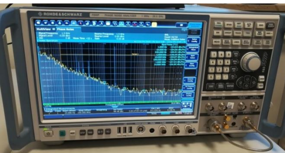
Settings: Additive Phase Noise Measurement/ Input Power 10dBm@1.3GHz/XCORR=1/no corr./ (2 channels)
