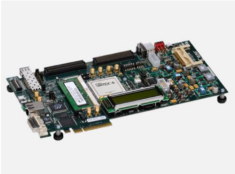
The digital control units in the Injector Linac are based on Xilinx ML605 and its daughter board.
