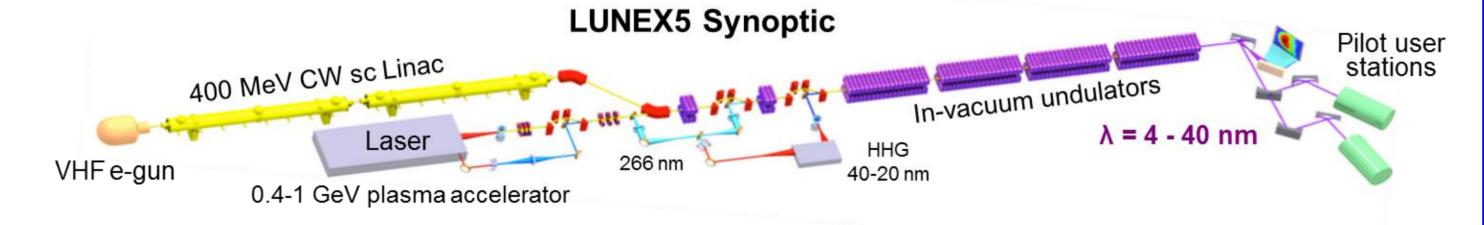
Phase 1: based on a 400 MeV CW sc Linac → explore advanced FEL techniques and applications
