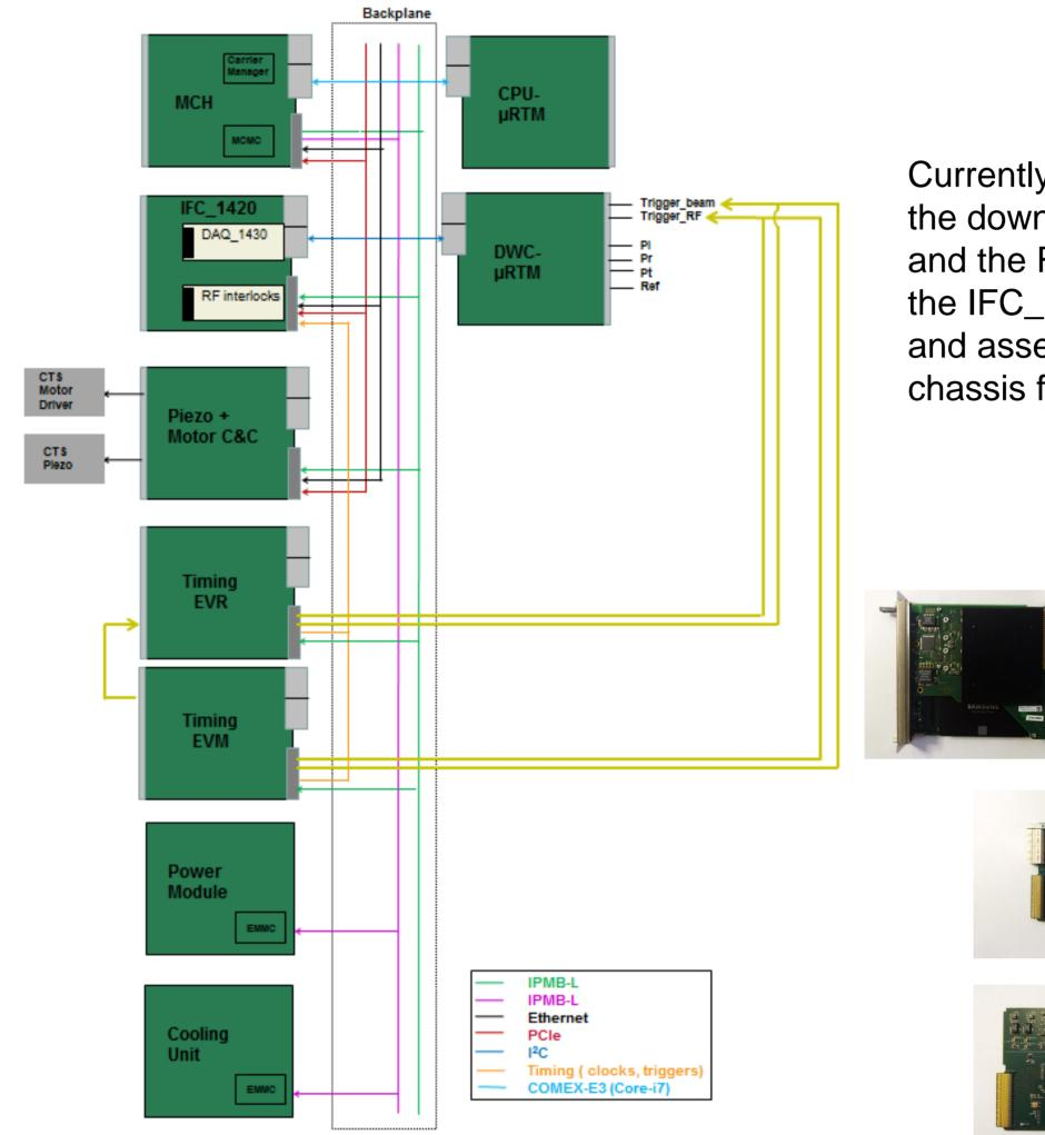
Currently, all the hardware, except the downconverter µRTM module and the RF interlocks (embedded in the IFC\_1420), has been acquired and assembled in a Native-R5 chassis from N.A.T.
