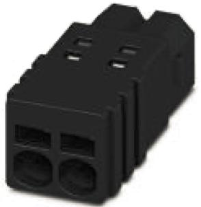
Plugs have small wedge-shaped protrusions that expand the receptacle body slightly when inserted. The protrusions lock into cut-outs in the receptacle body. Separation force is about 1 pound.
