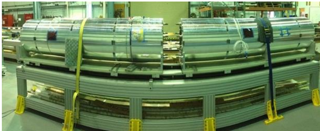
Fig. 6.19. “Panoramic” view of magnet integration table, shown with two half-length shell-yoke assemblies prior to joining.
