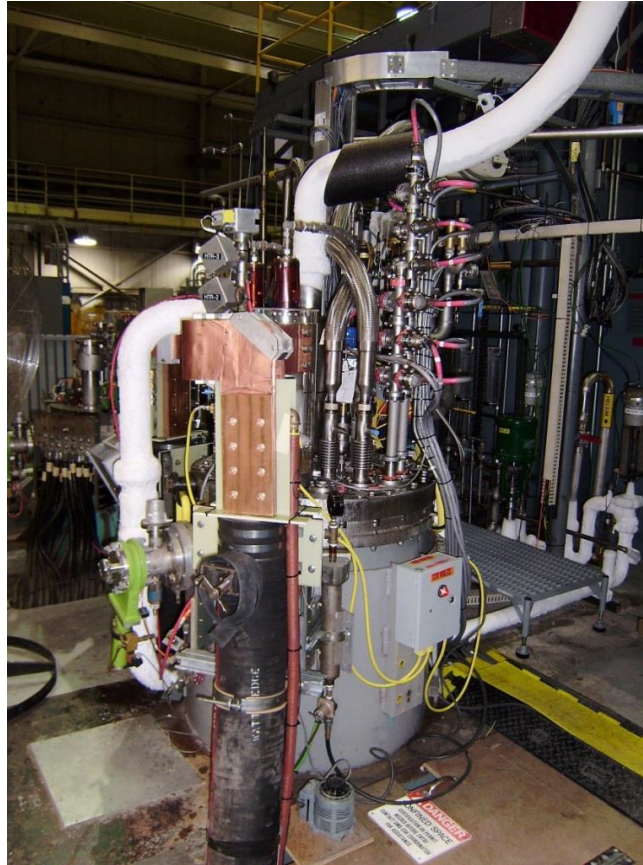
Figure 7.2: Vertical Test Stand 3, upgraded to provide 1.9 K at 1 bar (nom) and 24 kA, for testing of the 4.2 m-long MQXFA quadrupoles. The picture shows the test stand with the mirror MQXFPM1 under test.
