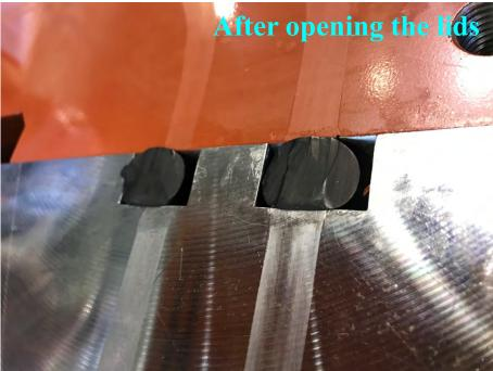
7) We installed new gaskets and cut the gaskets in such a way that the ends of gaskets were  $5 \sim 6$  mm above the surface of the cross member.
