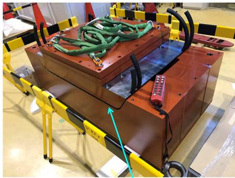
The cross member did not fit neatly into the main body and there was about 5 mm of gap between the cross member and the main body.
