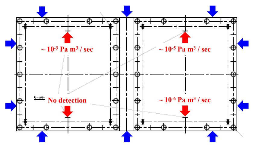
**From outside -> No detection** From leak test port (between gaskets) -> Detection (shown above)
