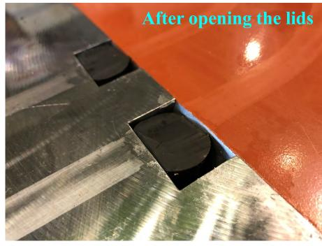
4) We cut the gaskets in such a way that the ends of gaskets were  $2 \sim 3 \text{ mm}$  above the surface of the cross member.
