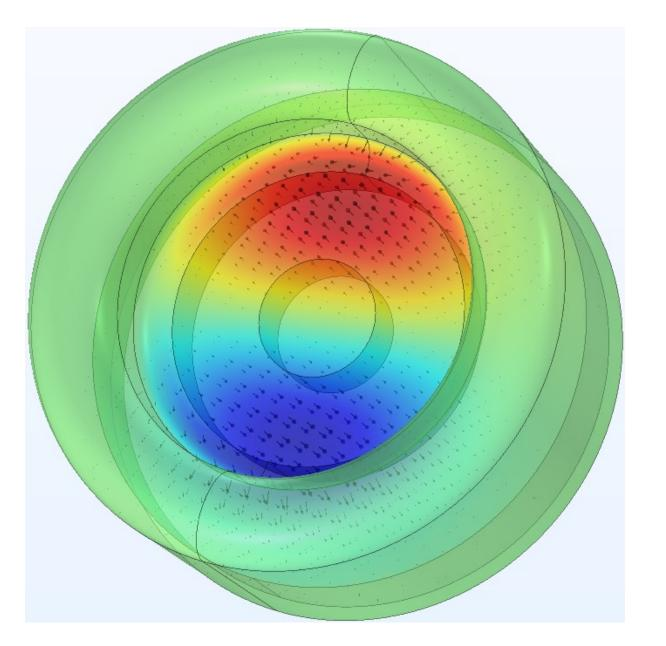
The pump optical mode  $(a_p)$  is driven to coherently couple the optical signal mode  $(a_s)$  with the microwave mode (b), with the electro-optic (EO) coupling strength g about  $2\pi \times 60Hz$ . The interaction Hamiltonian model this system is
