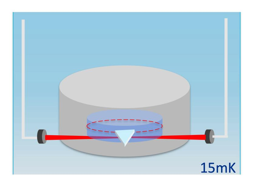
The 3D hybrid quantum system consists of a bulk Nb SRF cavity embedded with an optical made Lithium resonator of RF Niobate. The cavity supports a 9GH dipole mode. optical LN The resonator whispering gallery supports mode.
