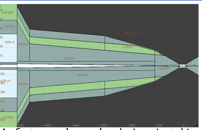
A first novel nozzle design is taking place. The aim is to reduce the BIB peaks modifying the shape and the composition of the nozzle profile.
