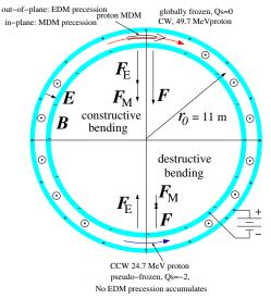
▶ The EDM signature is "out-of-plane" precession of the MDM
