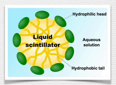
WbLS uses surfactants to form nm-scale micelles of liquid scintillator, such that a suspension can be formed.
