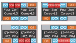
4 x 8-core Chiplet, 213mm 2 per chiplet 852mm 2 total area (+9.7%) 0.59x Cost
