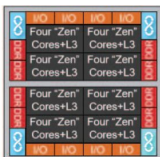
Monolithic 32-core Chip 777mm 2 total area 1.0x Cost
