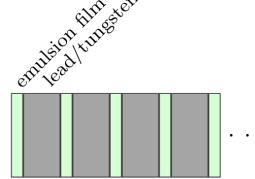
29 kg "suitcase size" prototype detector, 480 m from interaction point, for 12.2 fb<sup>-1</sup> in *pp* collisions at 13 TeV.
