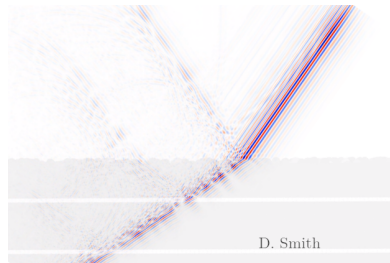
FDTD simulation of plane wave reflecting off a rough ice with under-ice layers:
