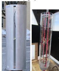
RNO-G quad-slot HPol (left), ARA VPol Bicone (right) :
