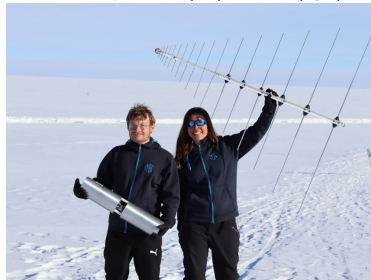
RNO-G quad-slot HPol (left), ARA VPol Bicone (right) :
