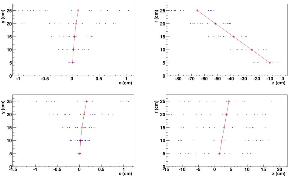
Trigger particle with  $p_T > 10$  GeV embedded amongst low  $p_T$  pileup tracks <sub>14</sub>
