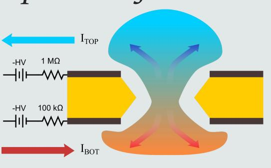
For larger area detectors, ohmic effects from protection circuits can dominate this by inducing currents through the protection circuits and reducing the gain
