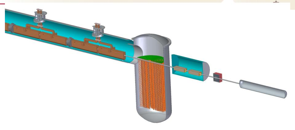
LN in boiler at same level as in cryomodules, covering Calrod array.
