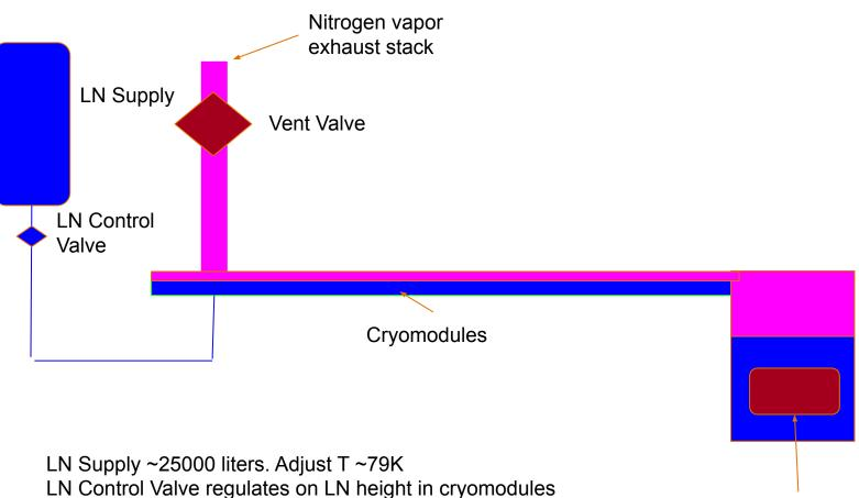
Vent Valve regulates on nitrogen vapor pressure
