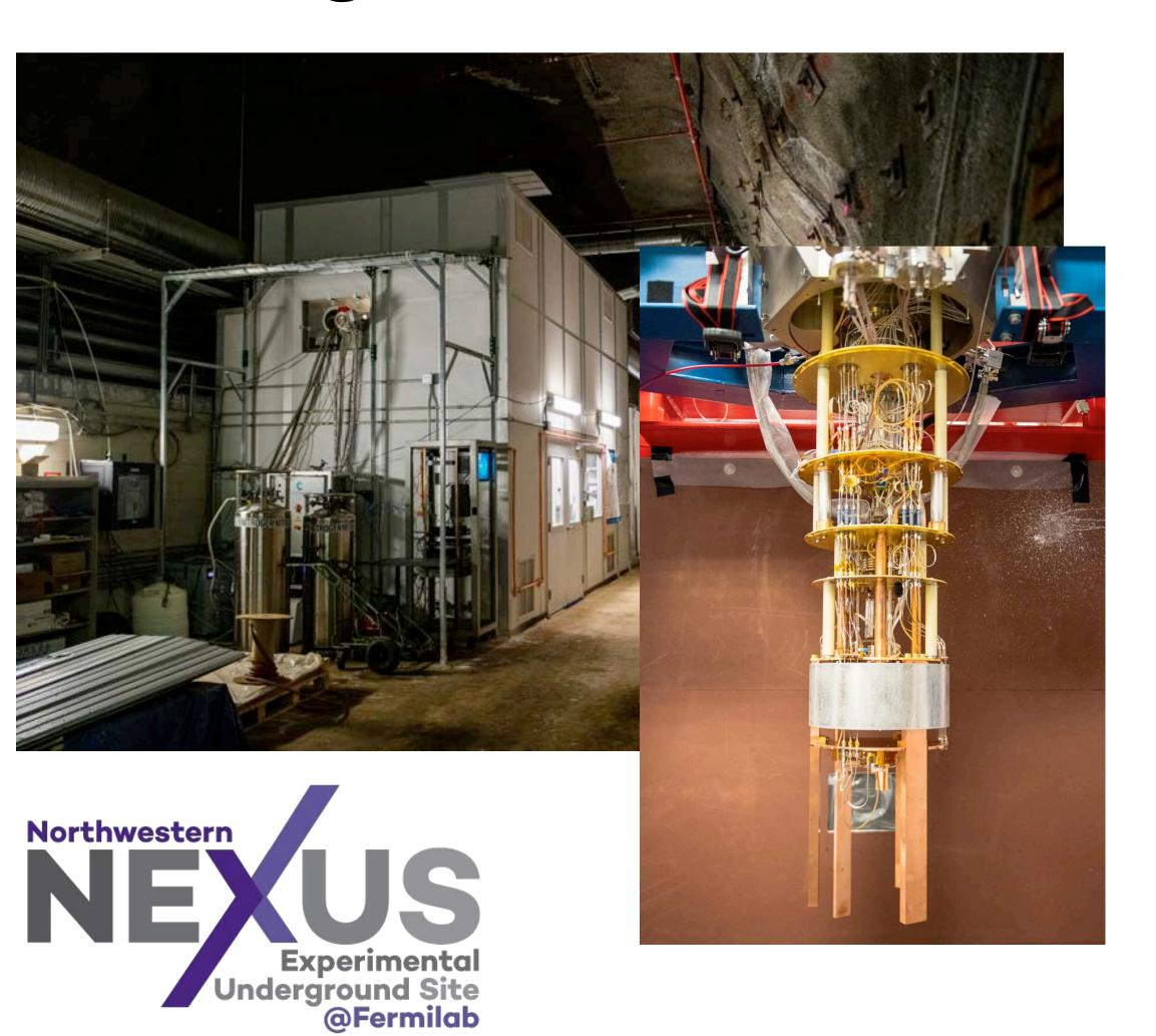
NEXUS multi-purpose low radioactivity cryogenic detector test facility
