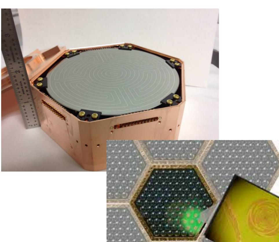
Bolometric detectors reach low thresholds with excellent energy resolution
