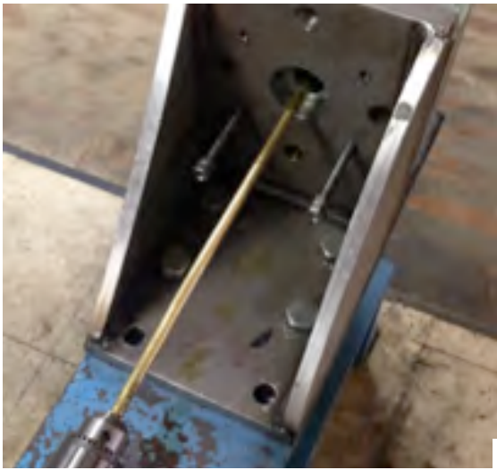
15 NbTi/Cu wires are cabled onto a perforated spring tube.
