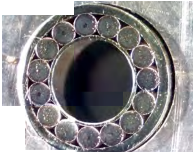
15 NbTi/Cu wires are cabled onto a perforated spring tube.
