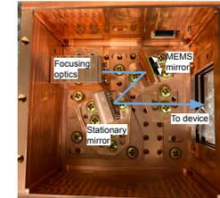
**Upper left:** Final design of scanning device, machined in copper
