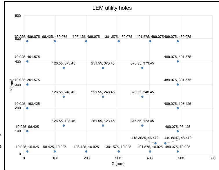
These positions will determine the location of dead areas due to utility holes when mapping signals to anode channels
