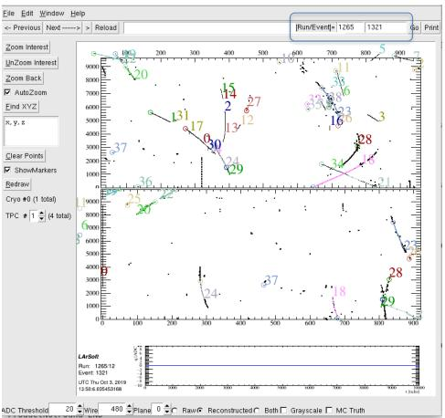
Many trajectories are broken up: missing hits due to LEM dead borders
