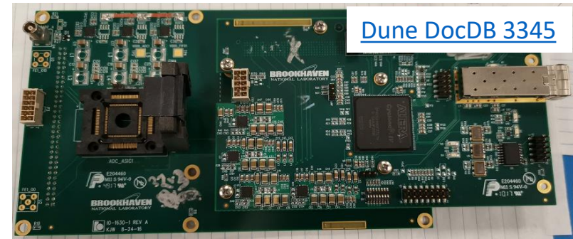
Single-socket ADC test board ADC Failure Mode
