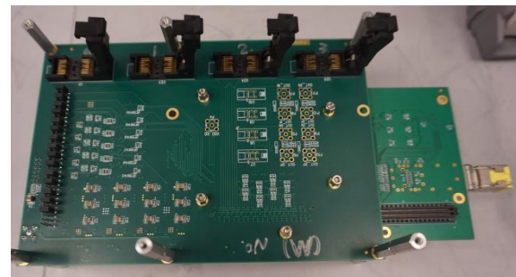
EPCS Cold Screening Test Board
