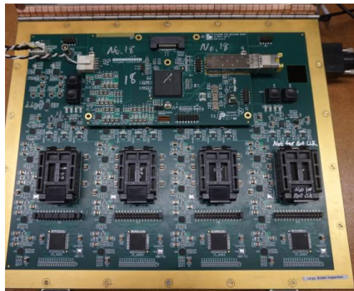
Quad Socket ADC Test Setup (RT)
