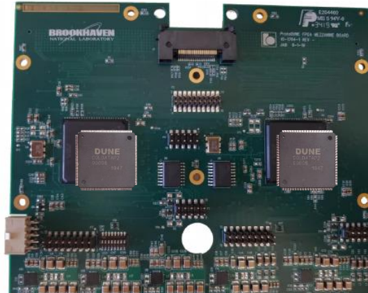
COLDDATA Mezzanine (FM)
