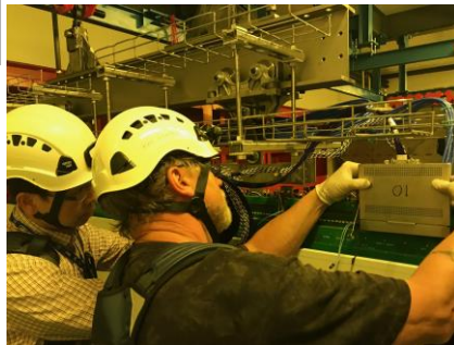
Manhong Zhao and Ken Sexton installing CE Box assemblies
