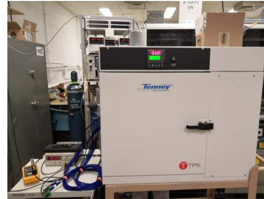
Temperature cycling in environmental chamber -65°C ~ 60°C
