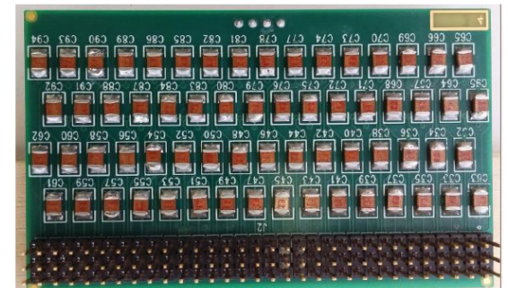
Toy TPC (150pF/120pF) (emulate detector capacitance)
