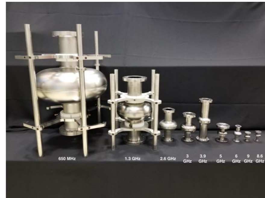
1-cell Fermilab cavities of various frequencies
