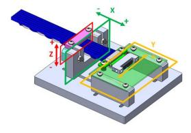
Done by Manhong Zhao at BNL: Redesigned connection between the cold control/data cable and the FPGA mezzanine board has been verified by mechanical fit check and temperature cycling tests and liquid nitrogen immerse tests.
