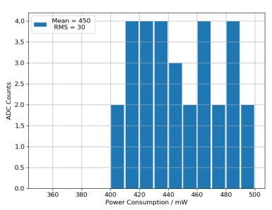
Power consumption at cold is ~40mW higher than warm in average (CMOS Reference, SDC&DB bypassed, single-ended inputs)
