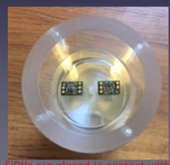
SiPMs are placed in contact with the BGO crystal
