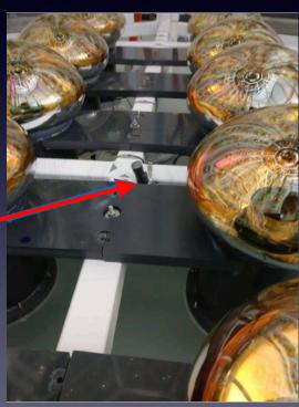
Bottom LED fibre placement
